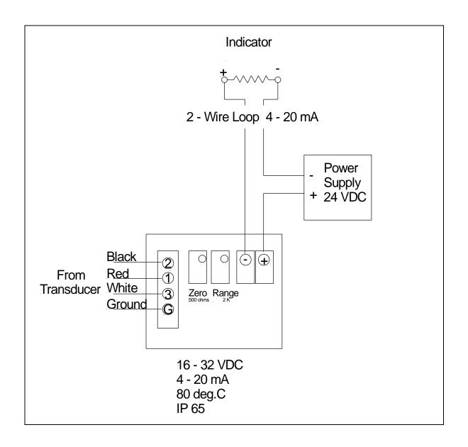
The XR 100 signal conditioner module is mounted onto a level transducer such as the SR series, which have a reed chain resistive output.
